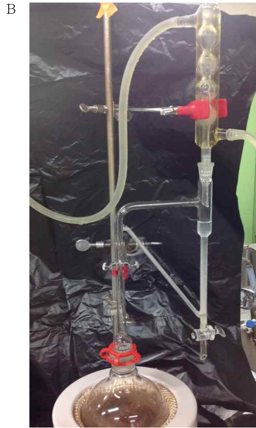
Fig. 54. Extraction method of essential oil by clevenger apparatus type.
