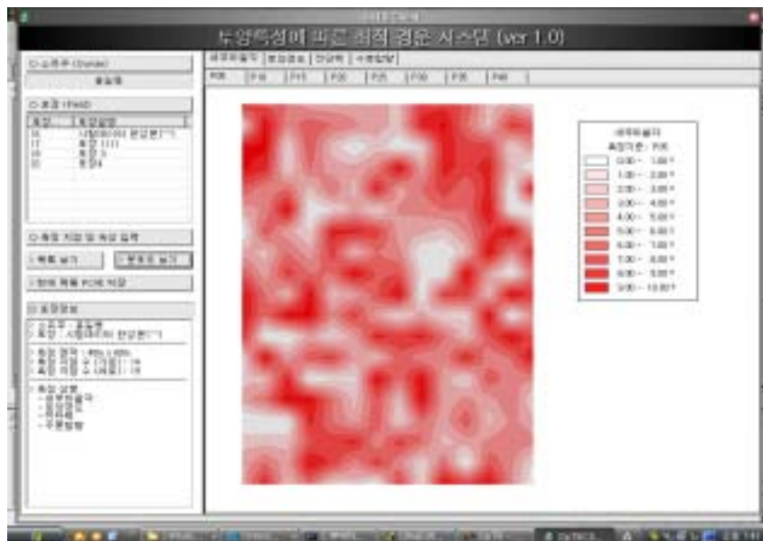
Fig. 43 An example of an attribute map interpolated by TIN method in 'Optill' program.
