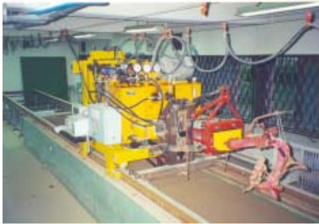
Fig. 13 Janggi with three point hitch and draft measuring system.
