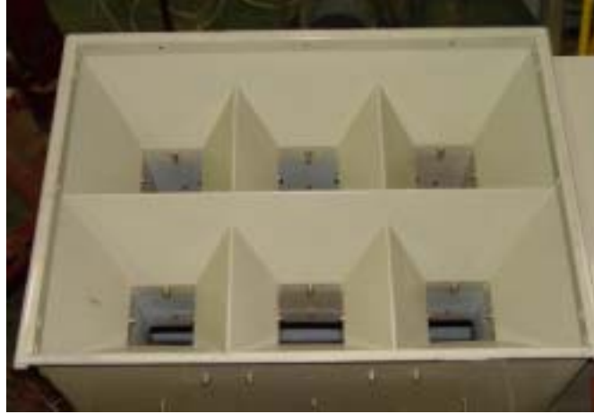
Fig. 3-11 View of rice inlet(Y-type chute).
