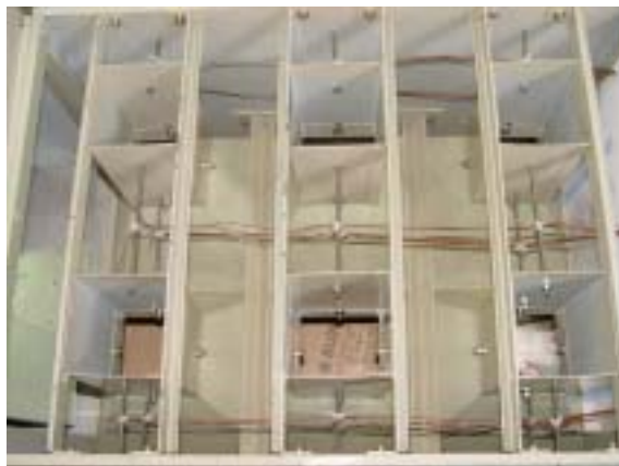
b) View of temperature sensor positions in hot air inlet
