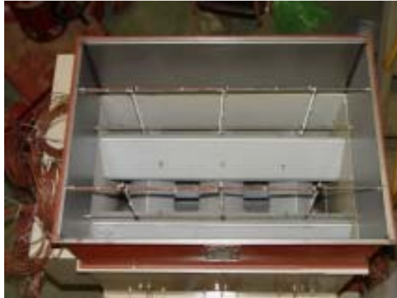
a) View of temperature sensor positions in drying section
