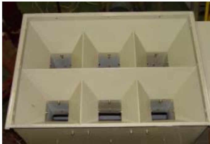
Fig. 3-32 View of rice inlet(Y-type chute).
