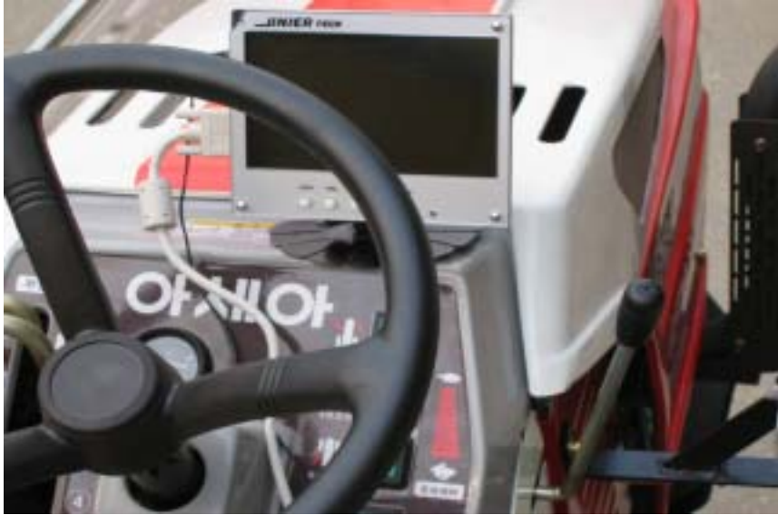
Fig. 5-63 The display part of variable-rate fertilizer controller
