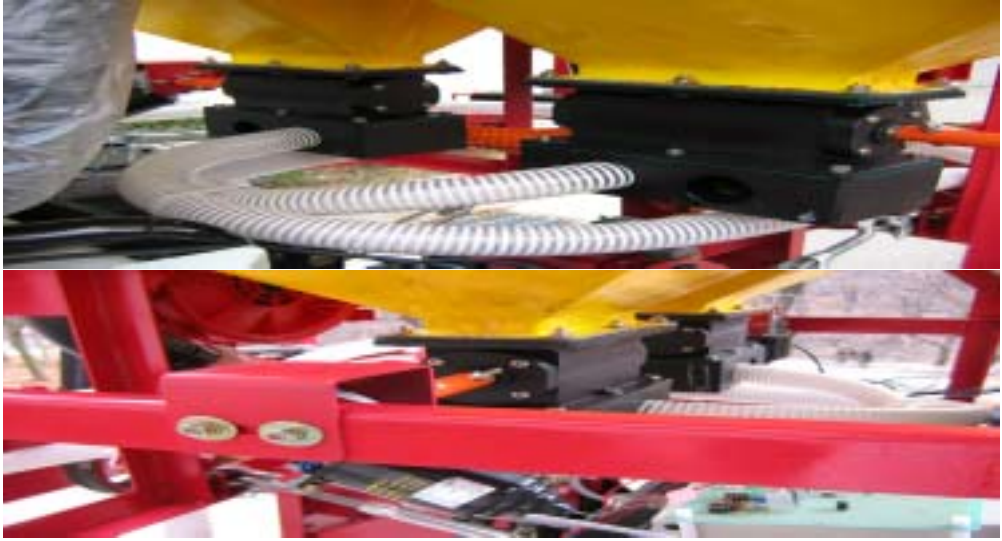
Fig. 5-59 The hopper which an granule discharge device is installed
