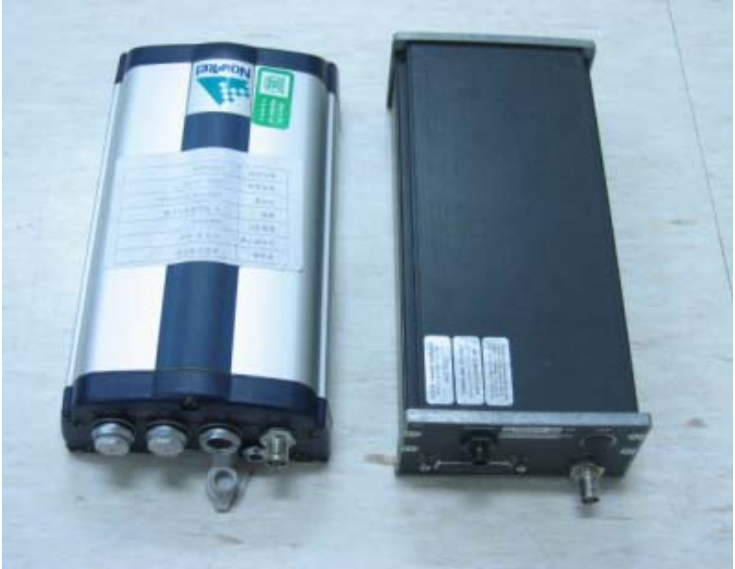
Fig. 5-107 GPS receiver and radio modem.
