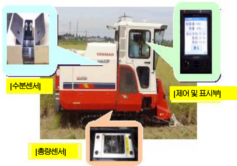
Fig. 3-2 Yield monitoring system for head-feeding combine (BRAIN in Japan)
