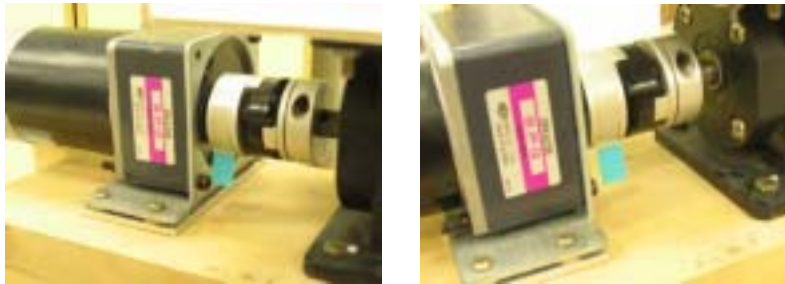
Fig. 5-60 Discharger which is adjusted to the motor using the flexible coupling
