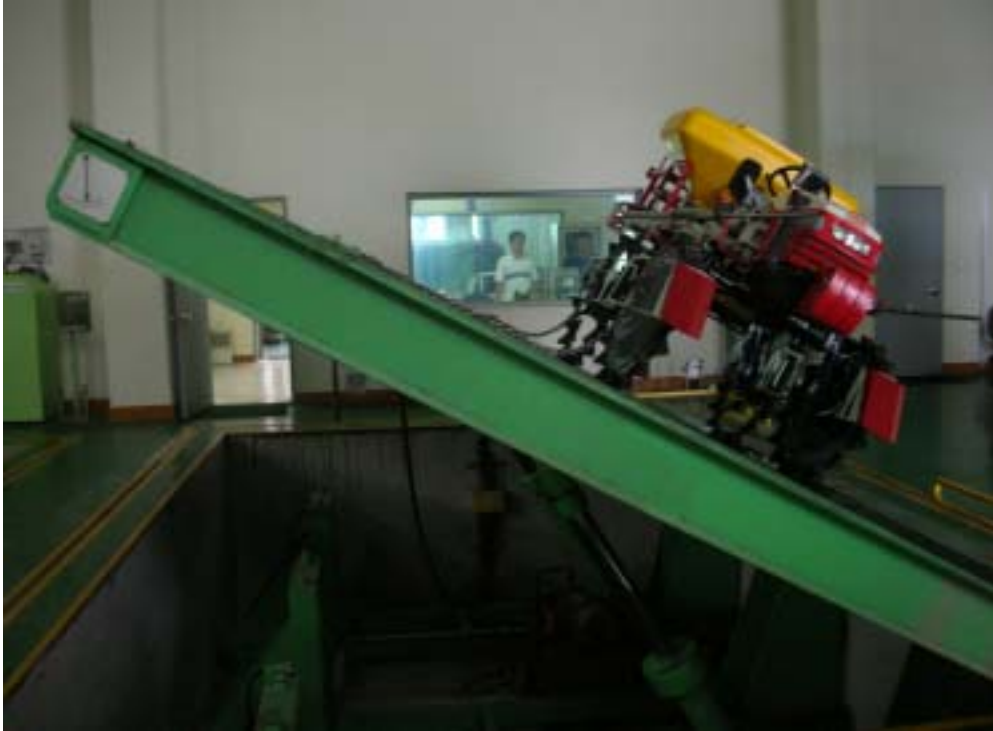
Fig. 5-125 View of measurement of angle static falling down sidelong
