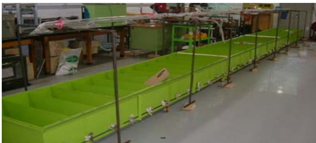
Fig. 5-26 View of fertilizer application patternator
