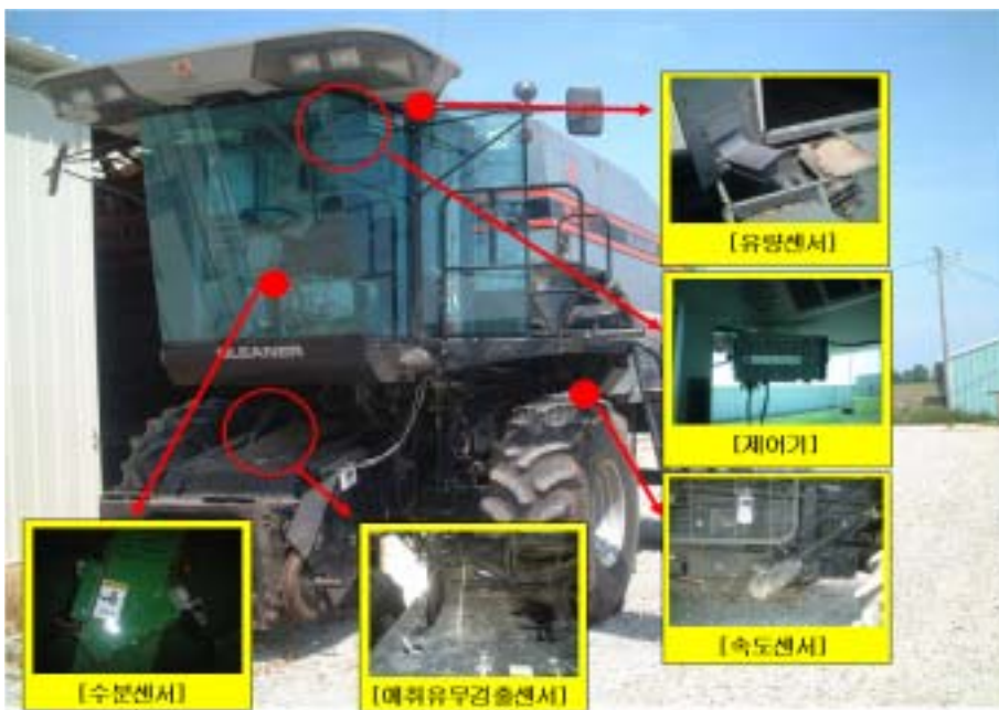
Fig. 3-1 Yield monitoring system using in U.S.A and EU
