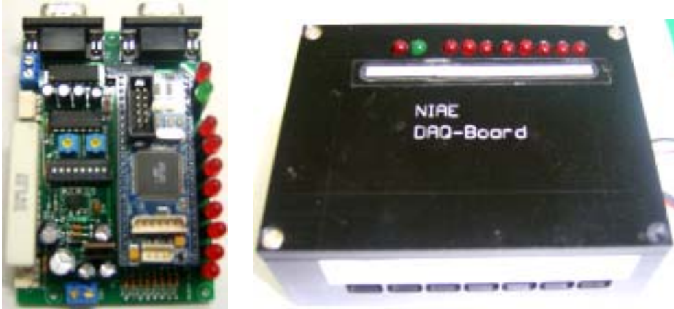
Fig. 3-42 Data acquisition board.
