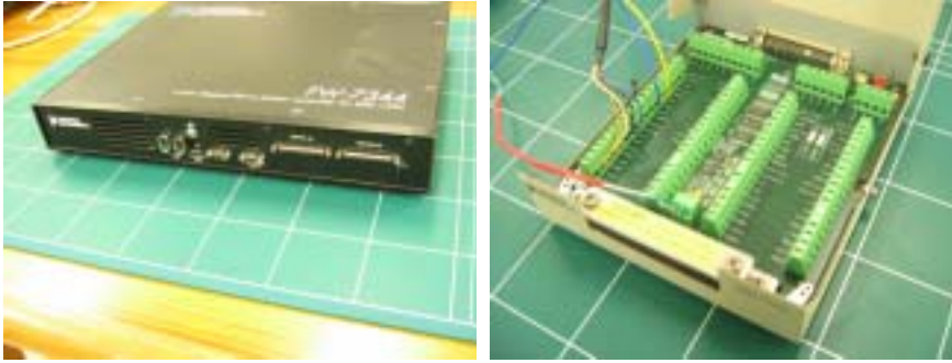
Fig. 5-58 The motion controller FW-7344 and UMI-7764
