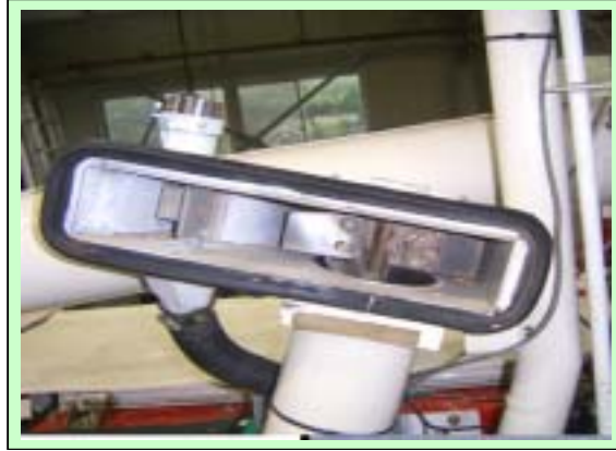
Fig. 3-7 Grain flow rate measuring sensor.
