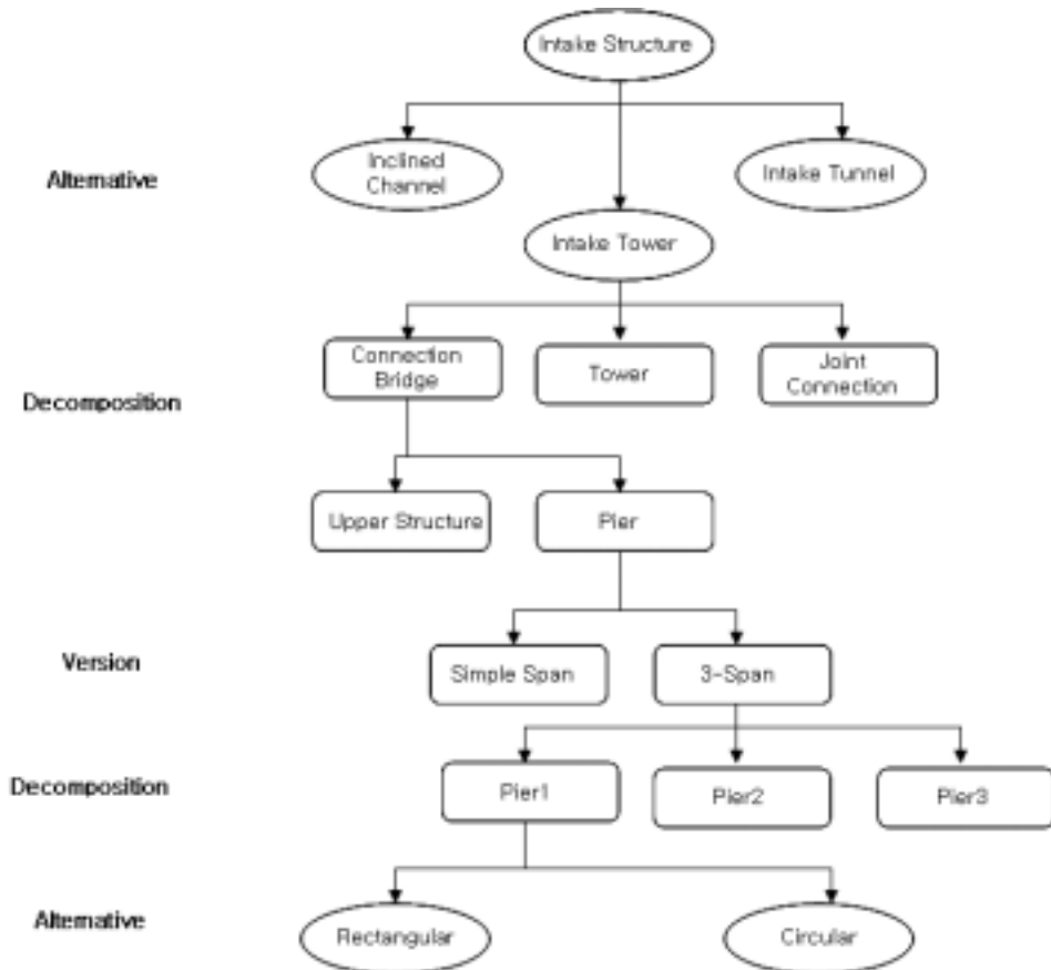
[Figure 3-85] Example of design object evolution in intake structure
