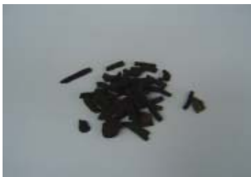
Fig. 38. Monolithic forms of adsorbents binding with water-soluble high molecular materials.
