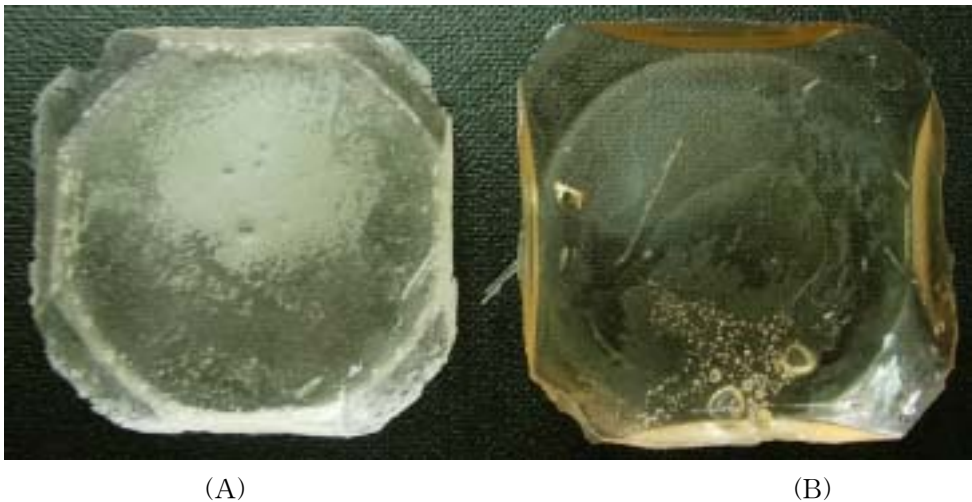
Fig. 39. Silicate film extracted by KOH (A) or by NaOH (B) from RHA500.
