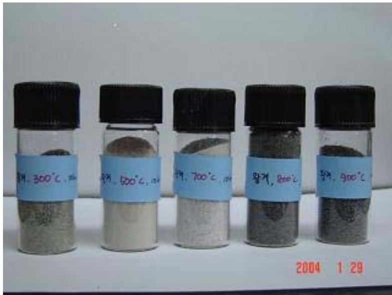
Fig. 5. The color of rice hull ashes; RHA300, RHA500, RHA700, RHA800 and RHA900.
