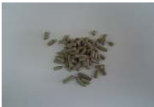
Fig. 38. Monolithic forms of adsorbents binding with water-soluble high molecular materials.
