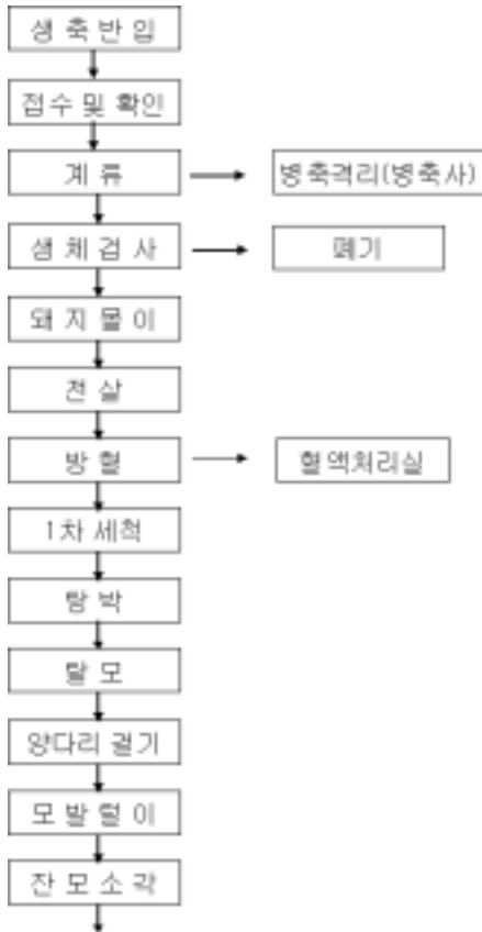
Fig 2-1. Flow diagram of slaughtering process
