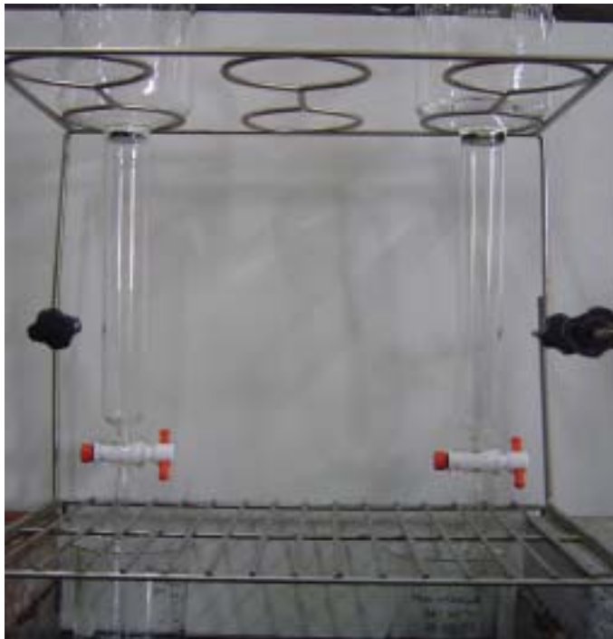
Photo 2-2. Flow tool for flow method using in release experiment
