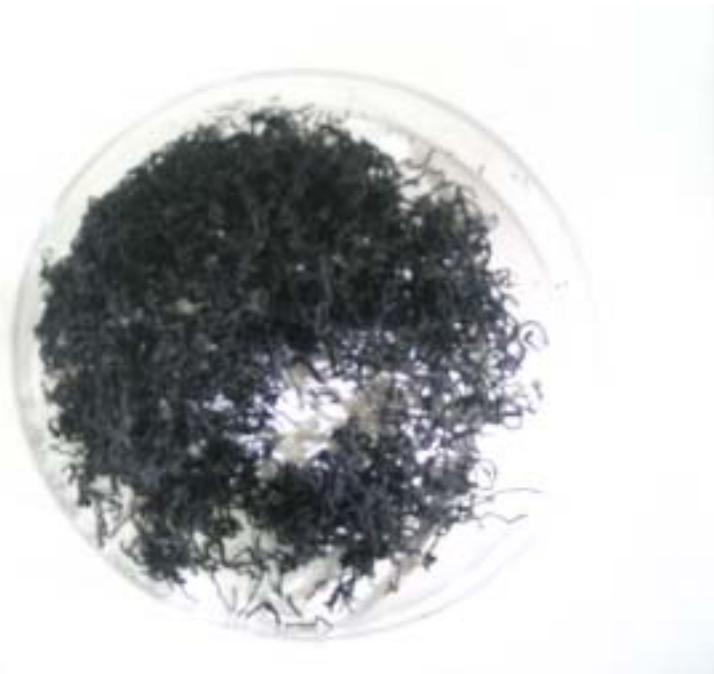
Fig. 3-25. Photograph of the immobilized malic acid degrading yeast cells with Korean oak charcoal and sodium alginate for the degradation of malic acid in wine.
