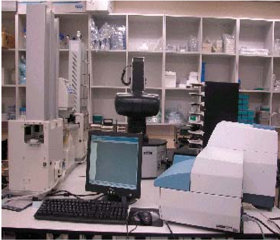
Fig. 3.4.3 The HTS system. A liquid handler, a multilabel counter and a robotic arm are integrated to each other.
