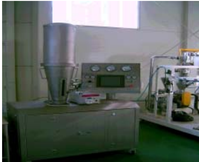
Fig. 1.11. Granulation apparatus including the main body, spray pump, and chamber.
