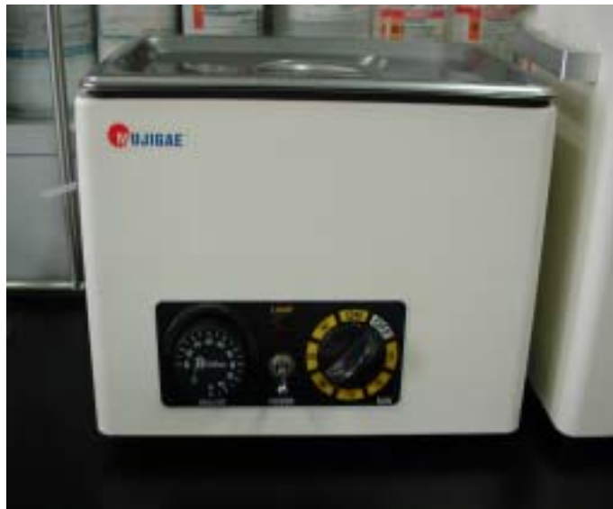
Fig. 2-8 28kHz ultra-sound apparatus
