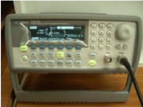
Fig. 3-17 A functional generator
