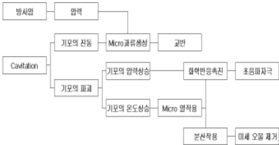
Fig. 2-1 Block diagram of the ultra-sound stimulus
