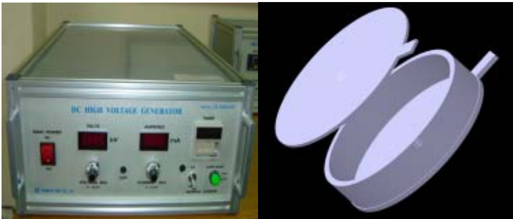
Fig.3-24 The apparent of A DC high voltage generator for the germination treatment of brown rice in the electrical field(left) and the sample container(right)
