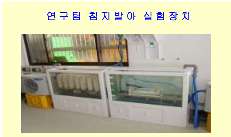
Fig.3-27 A soaking experimental apparatus for germination of brown rice
