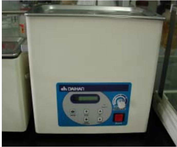
Fig. 2-9 40kHz ultra-sound apparatus
