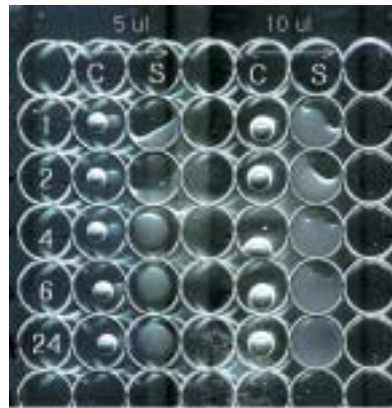
Fig. 2-38. 10W-40 Penzoil 에 coating 된 96well plate에서의 drop collapse 양상. C; negative control (LB broth), S; positive control.
