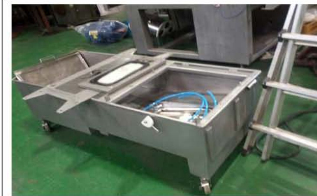
양념 tank & filter drum type
