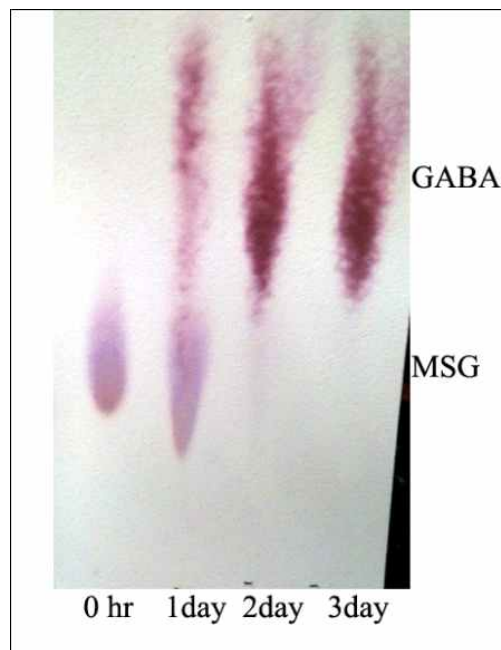
Fig. 33 Scale up of GABA production by 75L fermenter using L. brevis G100 and the extract of Gastrodia elata
