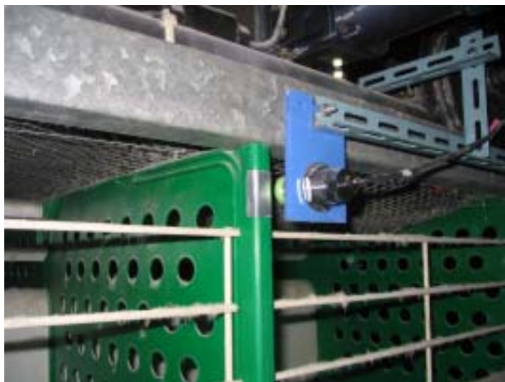
Fig. 18 A view of a proximity switch and a sensing plate.
