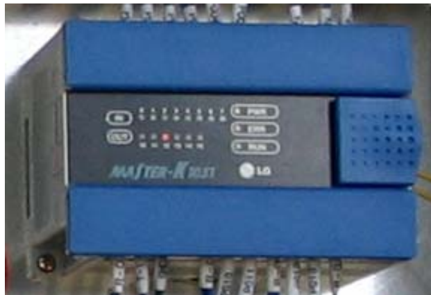
Fig. 51 A view of PLC(Programmable Logical Controller).
