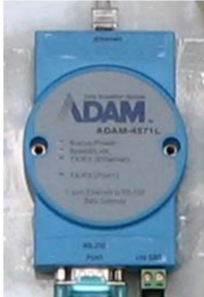
Fig. 53 A view of RS 232 to Ethernet data converter.
