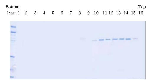
Fig.6. Polypeptide of viral coat protein in SDS-PAGE. Analysis showing the distribution of the viral coat protein following equlibrium centrifugation in 50%(1.585g/cm) cesium chloride. Viral coat protein were denaturated for 5 min at 95°C in 50Mm Tris-Cl, pH 6.8, 100mM dithiothreitol, 2% SDS, 10% glycerol, and 0.1% bromophenol. Denatured proteins were separated by 12% polyacriylamide gel electrophoresis. Gel was stained with Coomassie Brilliant Blue R-250.
