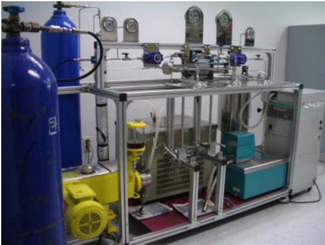
Fig3-1 Apparatus for supercritical carbon dioxide extraction
