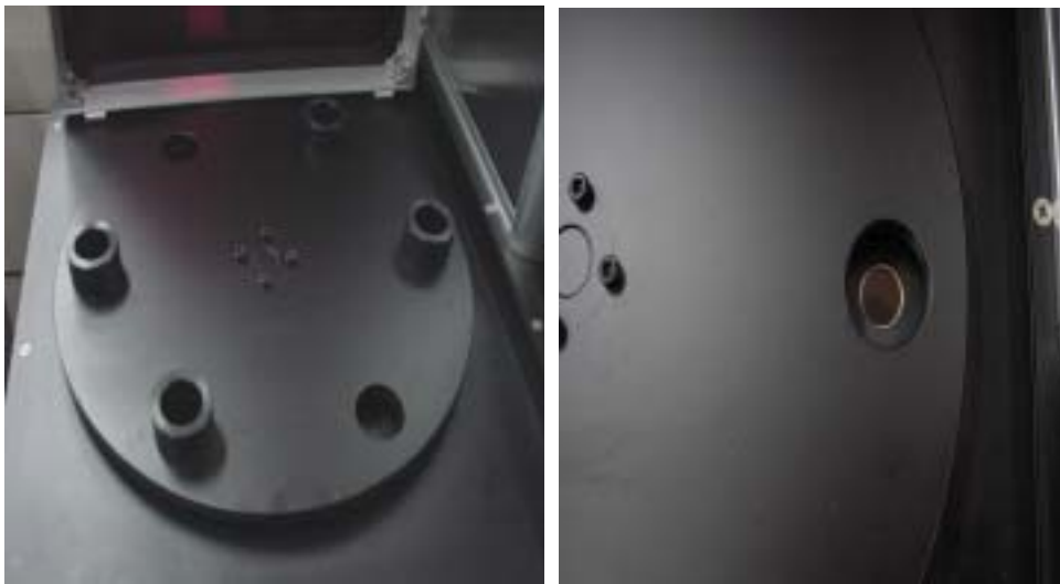
Fig 3-37 The view of rotating plate and photosensor window of Compost Quality Autoanalyzer
