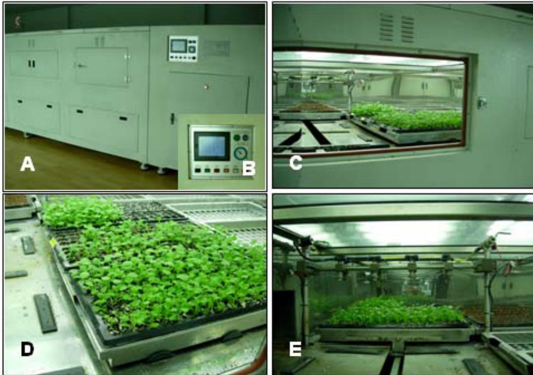
Fig 3. Parts of an Automatic Culture Chamber A. main chamber, B. digital control panel, C. retractable window, D. conveyor with plug trays and E. misting system for water and nutrient solution application.
