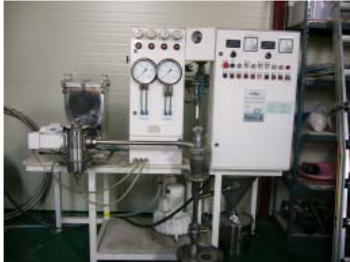
Fig. 1. Jet mill and air-classifying system
