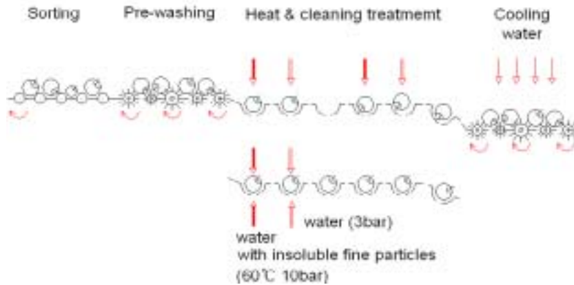
Fig. 3-7-7. Schematic of pressured mild hot water with insoluble fine particles treatment system for apple
