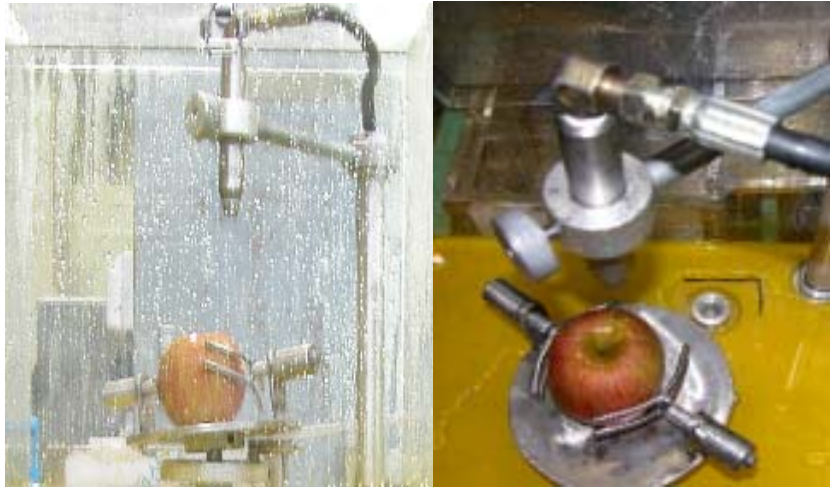
Fig. 3-7-4. Experimental apparatus of pressured mild hot water treatment system for apple
