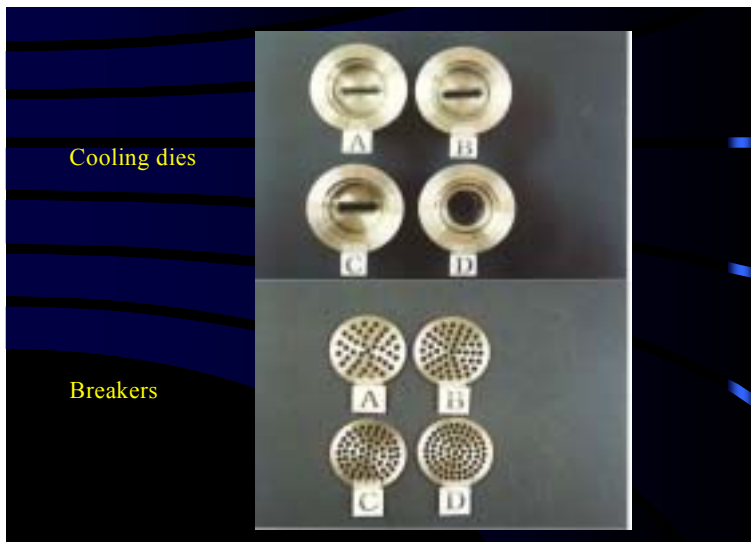
Fig. 1. Front View of Cooling Die and Bleaker Plate
