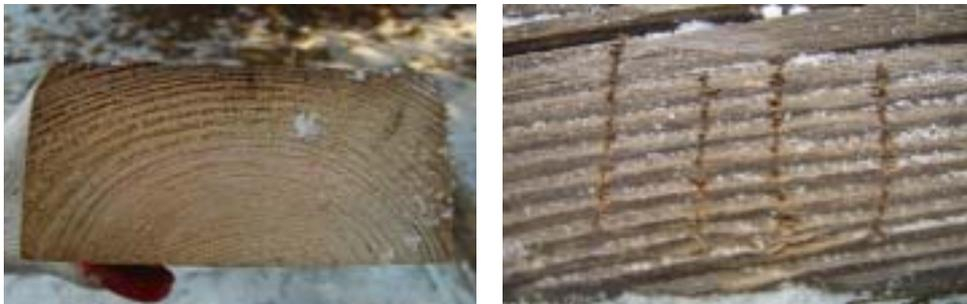
**Fig.4. Typical soft rot damages observed in dismantled wood members of old wooden building.**
