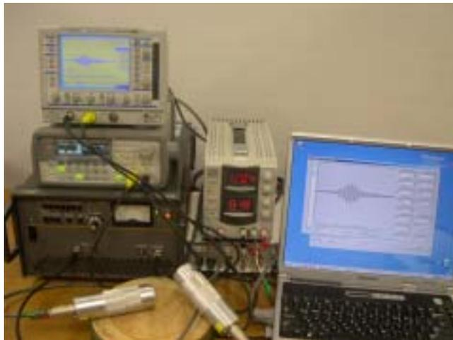
Fig.1. Ultrasonic test set up for measuring the transmission time of wave
