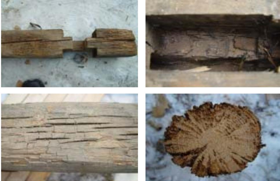
**Fig.3. Typical decay damages observed in dismantled wood members of old wooden building.**
