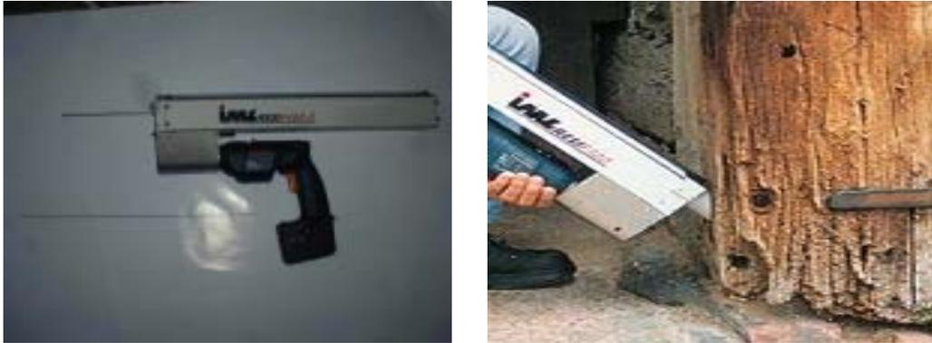
Fig13. The device of drilling resistance(IML-RESI).
