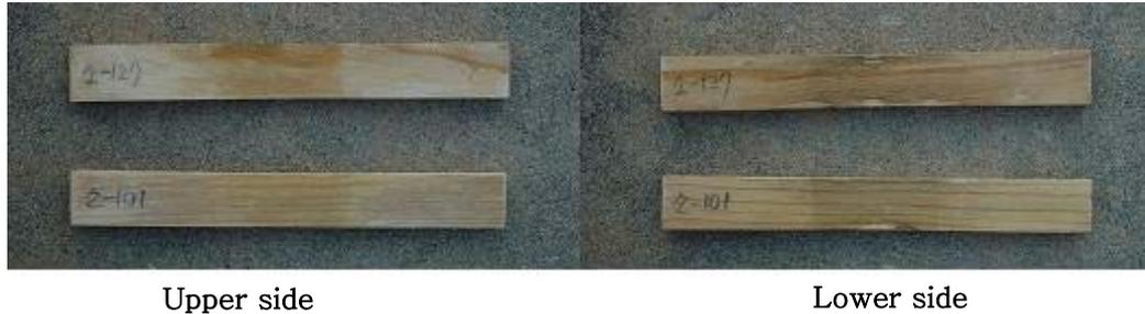
**Fig.28. Differences in decay area between upper and lower side of specimen attacked by *Fomitopsis palustris*.**
