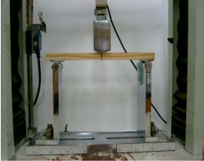
Fig. 4-1. Static bending test for spruce and pine elements by UTM.
