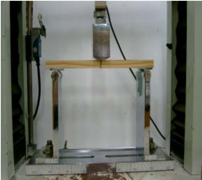
Fig. 4-5. Static bending test for spruce and pine elements by UTM.
