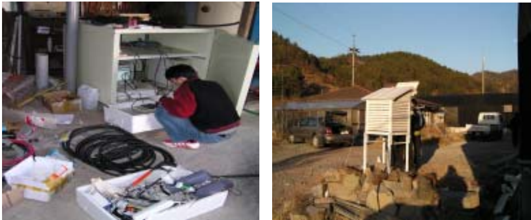
Photo 2-12. View of setting of measuring instrument and instrument shelter.
