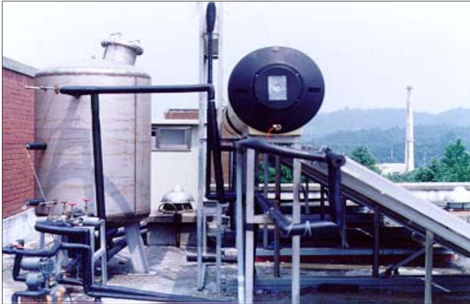
Photo 2-19. View of experimental equipment for forcedly circulated solar collector system.
