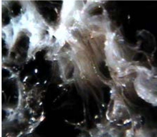
<그림 2-47> Micrograph ( \times 500 ) of the tensile fracture surface of liquefied wood polymer alloy prepared with LW : PE (10 : 90).
