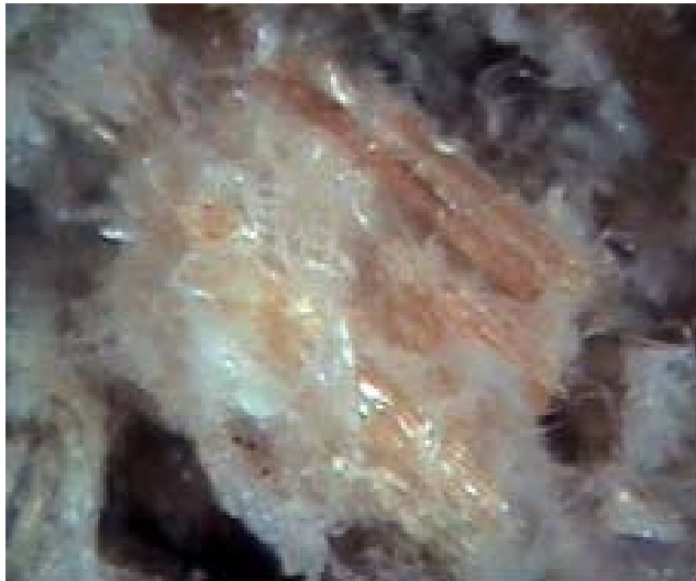
<Fig. 1-95> Micrograph ( \times 500 ) of the tensile fracture surface of wood flour polymer composite on WF treated with 3 day ammonia.
