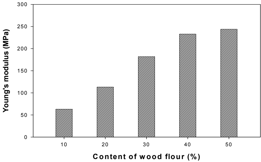
<Fig. 1-59> Young's modulus of wood flour polymer composite on WF
