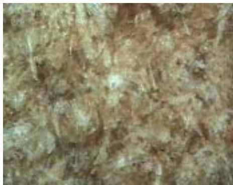
<Fig. 1-87> Micrograph ( \times 100 ) of the surface of wood flour polymer composite on WF content.
