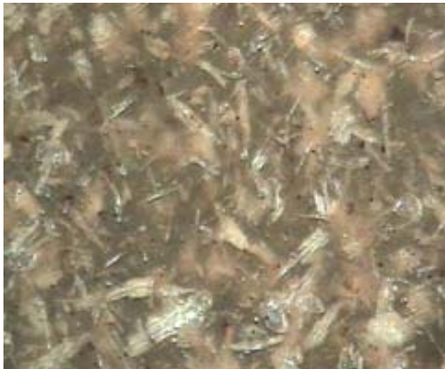
<Fig. 1-91> Micrograph ( \times 100 ) of the surface of wood flour polymer composite on esterified WF with PA 50%.
