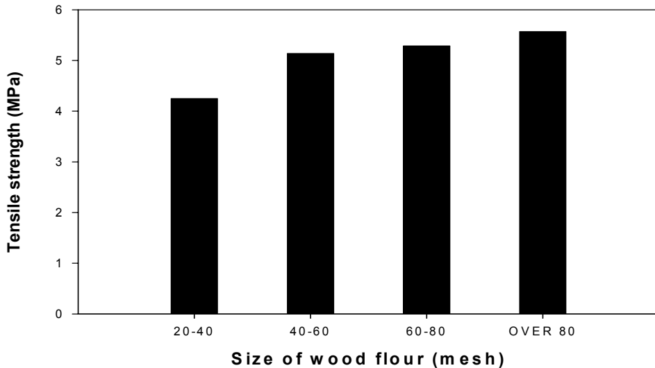
<Fig. 1-53> Tensile strength of wood flour polymer composite on WF size.
