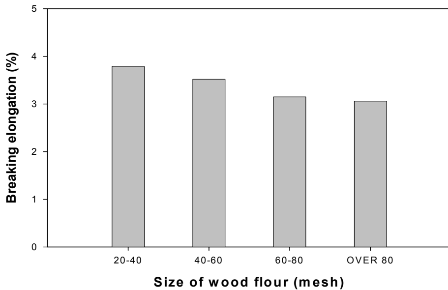
<Fig. 1-55> Breaking elongation of wood flour polymer composite on WF size.
