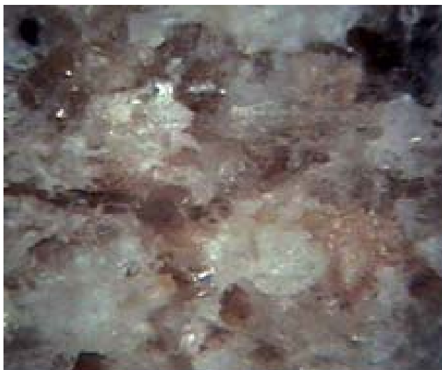
<Fig. 1-97> Micrograph ( \times 500 ) of the tensile fracture surface of wood flour polymer composite on esterified WF with MA 50%.
