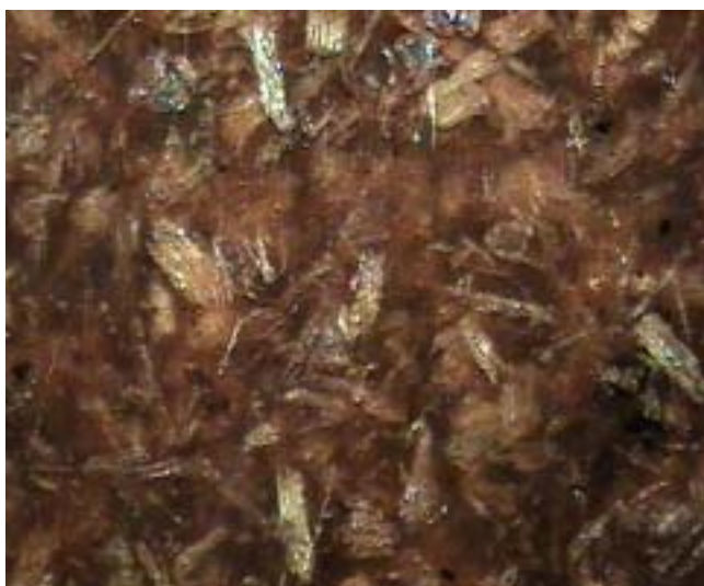
<Fig. 1-88> Micrograph ( \times 100 ) of the surface of wood flour polymer composite on WF treated with 3 day ammonia.
