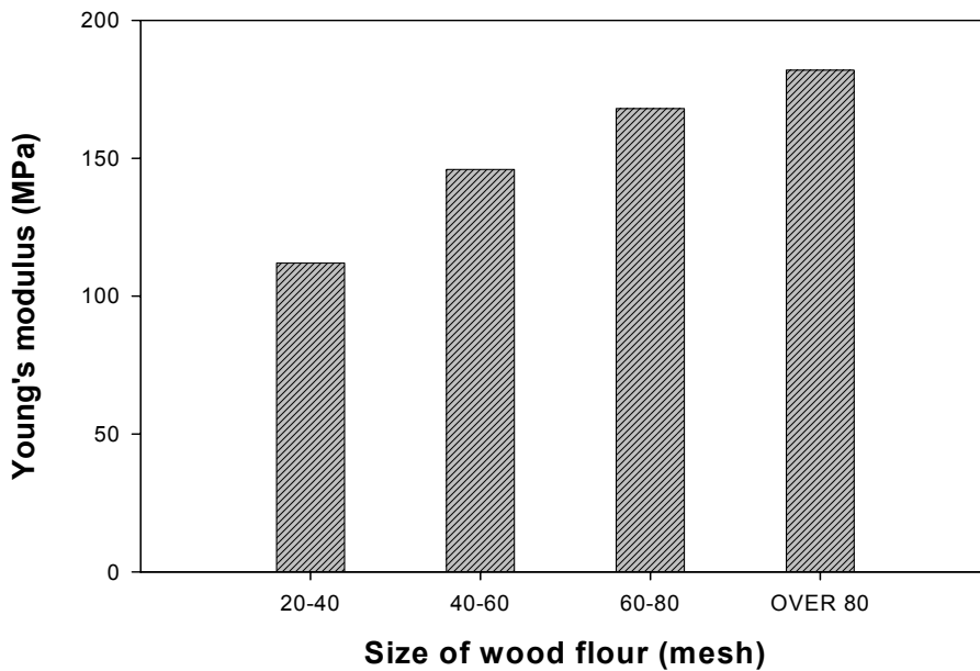
<Fig. 1-54> Young's modulus of wood flour polymer composite on WF size.
