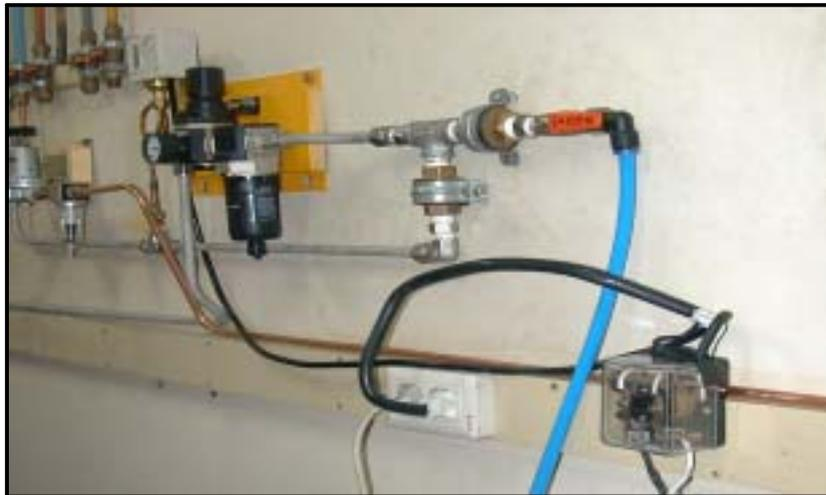
Fig. 42. Automatic safety system for air supply for 15L bioreactor.
