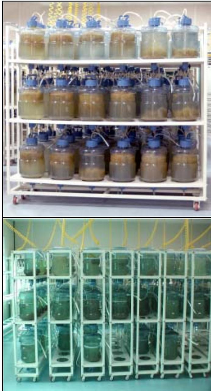
Fig. 43. Mass production of adventitious roots of *D. nipponica*. Upper: one set of 15L bioreactors (18 x 15L bioreactor), Lower: Multi-sets of 18-bioreactors(10 x 18 x 15L bioreactors, 2.7 ton)
