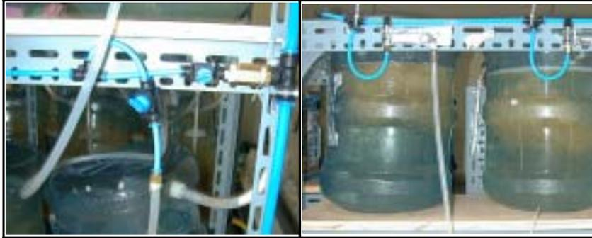
Fig. 41. Direct air distributor for multi-connection 15L bioreactors.
