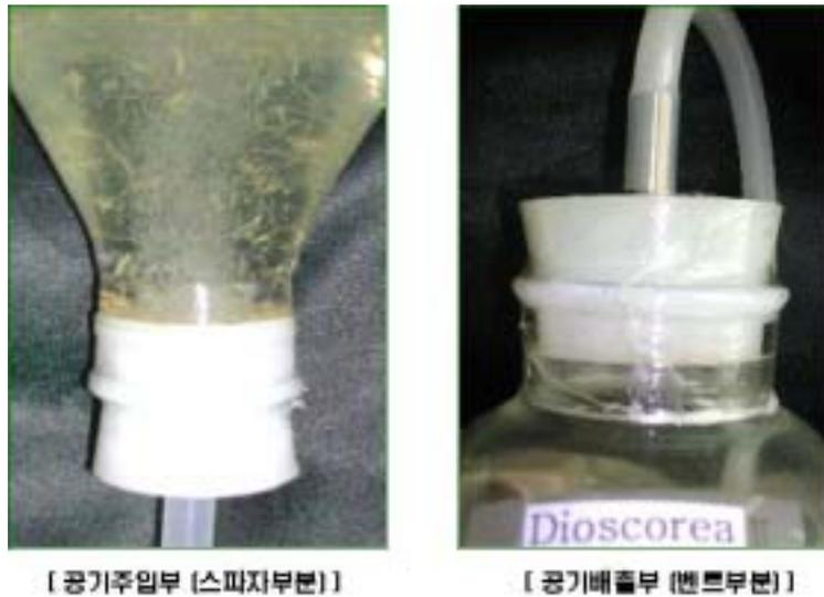
Fig. 27. Sparger and ventilation system of 2 L air-lift bioreactor.
