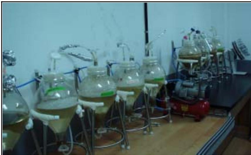
Fig. 33. Multi-connection culture by one air compressor for 5L glass type air-lift bioreactor used for culture of adventitious roots.
