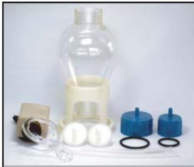
Fig. 31. Modified 2L air lift type bioreactor with plastic material.
