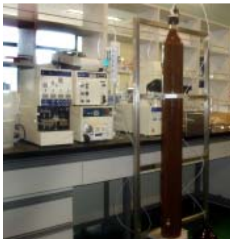
Fig. 86. MPLC with Dowex 50 x 8, Amberlite IRA-410 resin (20L)
