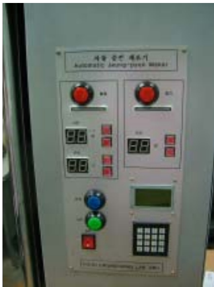
Fig. 5-33. Picture of finished JAS controller
