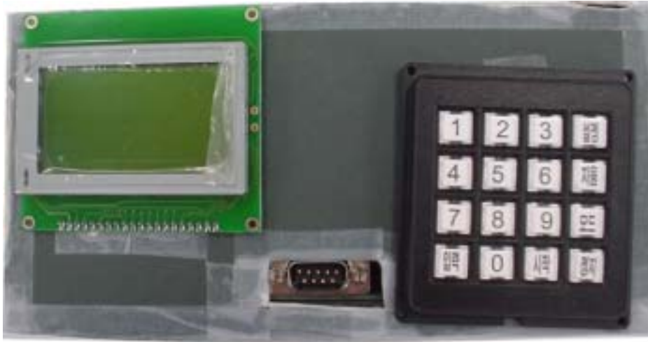
Fig. 5-15. LCD and keypad of finished Jeung-pyun controller
