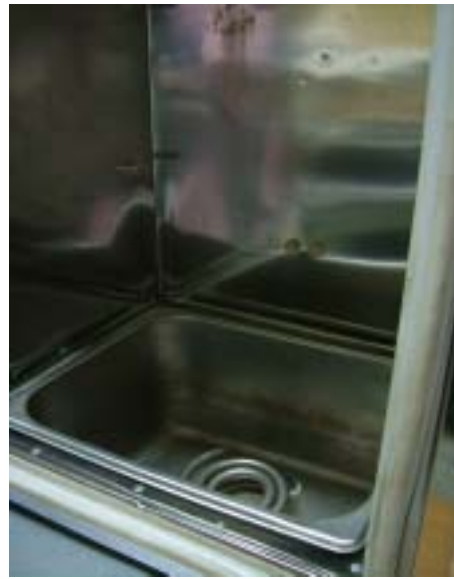
Fig. 5-32. Picture of finished steaming chamber
