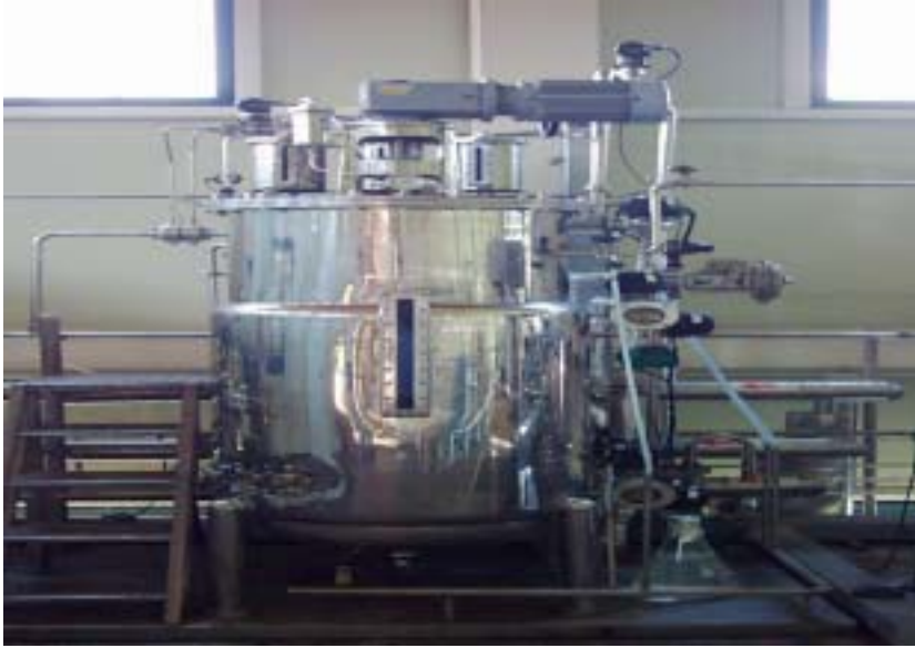
Figure 6. Submerged-liquid culture of Agaricus blazei in the 500 ℓ fermenter.
