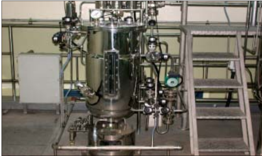
Figure 5. Submerged-liquid culture of Agaricus blazei in the 50 ℓ fermenter.
