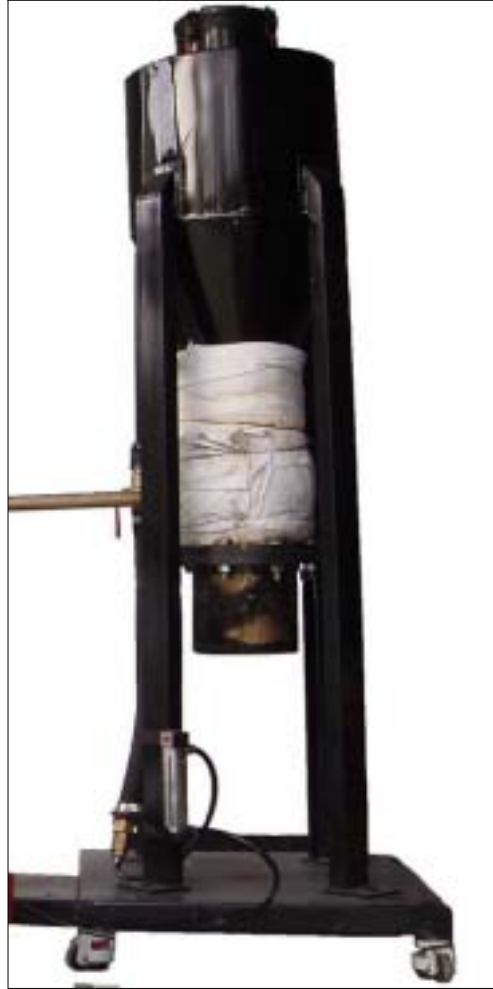
[Photo 3-18] Picture of Down-draft Gasifier Version.2
