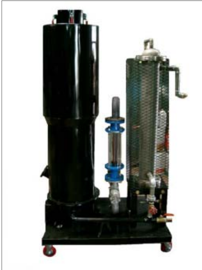
[Photo 3-17] Picture of Down-draft Gasifier Version.1
