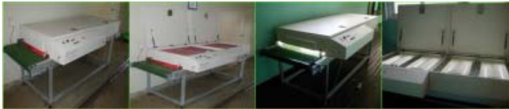
Photo. 2. The automatic conveyor system combined light treatment and drying, and the modified system using fluorescent light.
