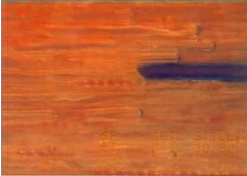
Fig. 34. Liquid penetration at a tracheid and ray crossing showing the liquid meniscus
