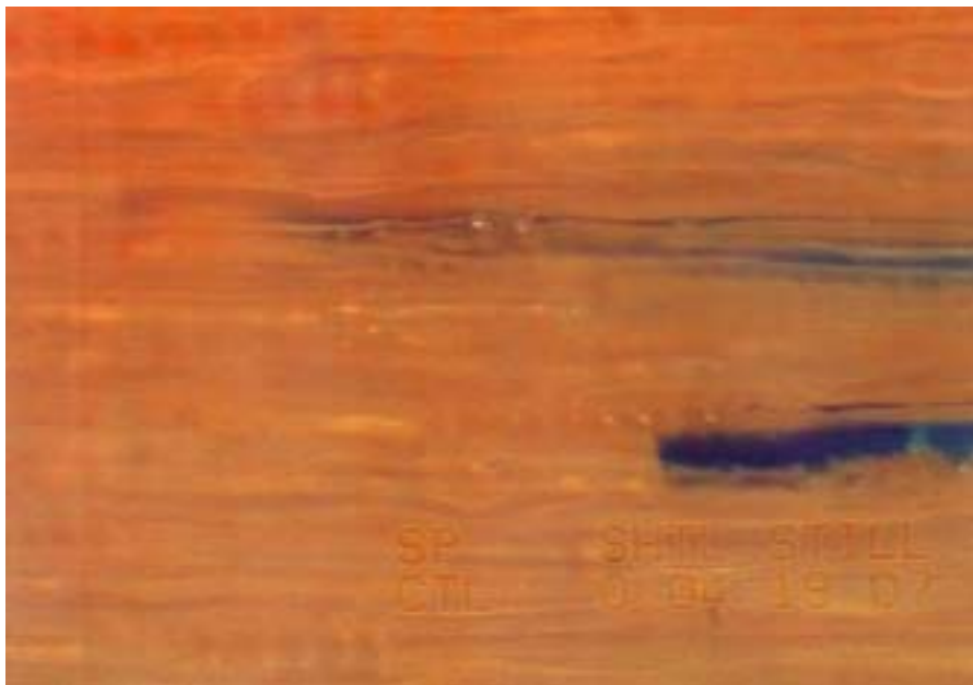
Fig. 33. Two stagnation position of liquid penetration. Upper. overlapped top position. low. Narrow tracheid lumen passed by ray.
