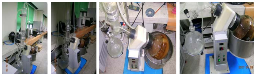
Fig. 12. Pilot system for extraction of high concentration and high yields of ITCs from horseradish.
