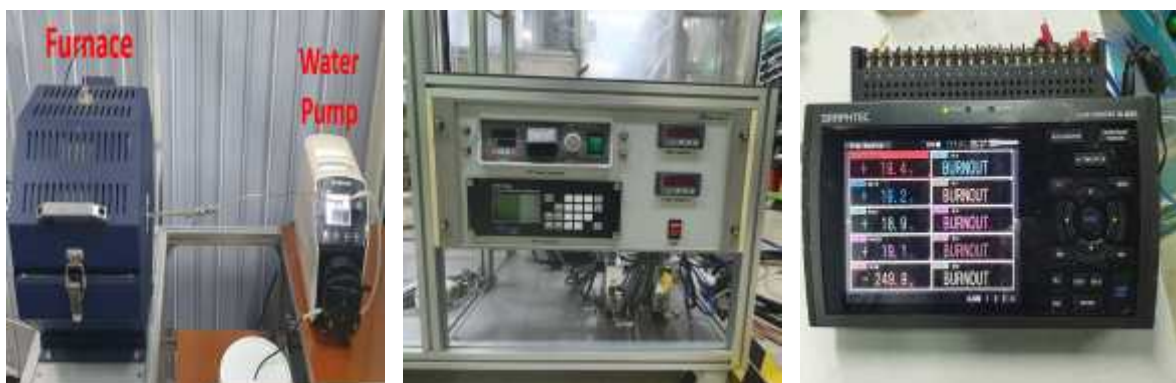
(a) Steam generator (b) Controller (c) Data logger
