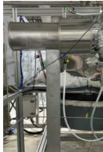
(f) Heat Exchanger
