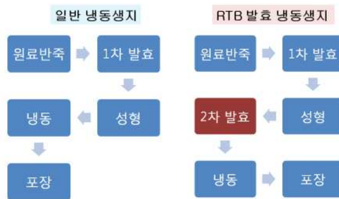
Figure 1. Comparison of manufacturing process between frozen dough and RTB fermented frozen dough
