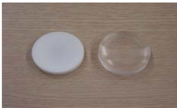
Fig. 3-9. Photo of fabricated wear plates with acrylic and Teflon.
