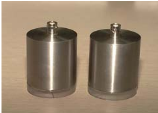
Fig. 3-31. Fabricated ultrasonic transducers with acrylic wear plate.
