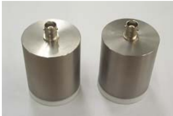
Fig. 3-34. Photo of fabricated ultrasonic transducers with Teflon wear plate.
