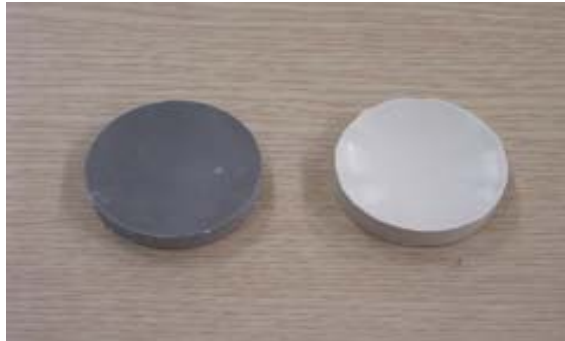
Fig. 3-8. Photo of fabricated wear plates with silicon rubber and tungsten powder.
