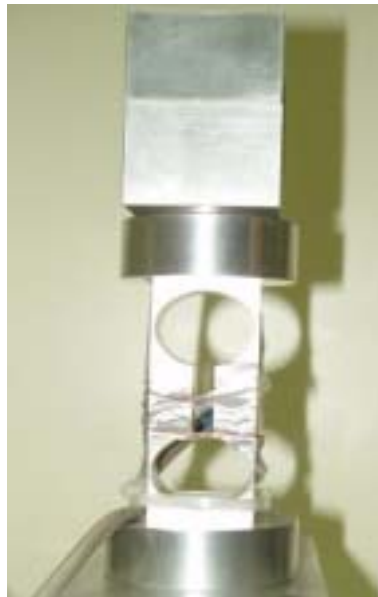
Fig. 5-6. Load cell mounted on the RX transducer.
