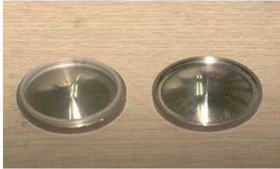
Fig. 3-7. Photo of zig with curvature for wear plate.
