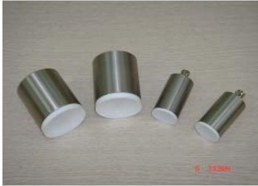
Fig. 3-47. 100 kHz and 200 kHz of the fabricated ultrasonic transducers.
