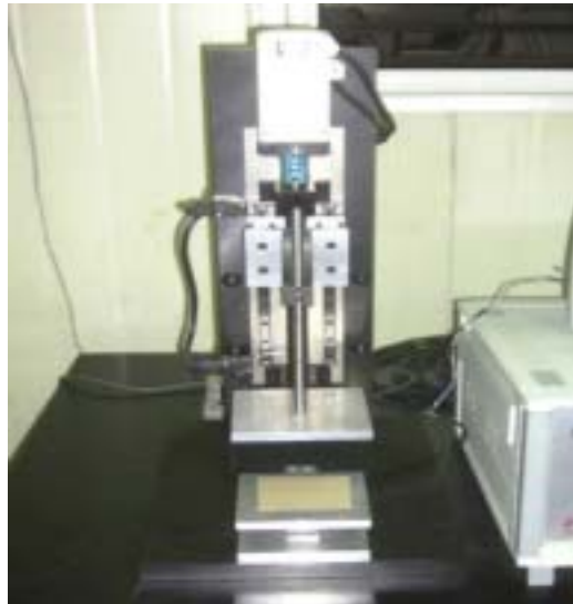
Fig. 2-36. Compression test apparatus for apple flesh specimen.
