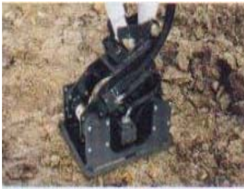
Fig. 44 View of compactor
