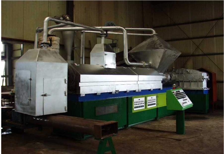
Fig. 3-6-7 Electric heater type waste vinyl recycling facility
