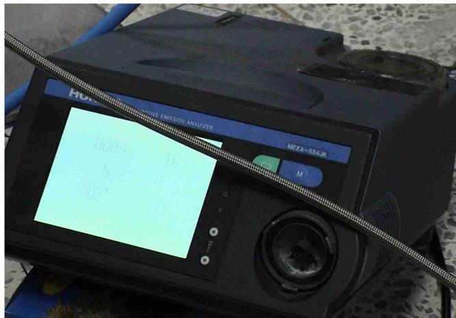
Fig. 3-5-19 Gas analyzer
