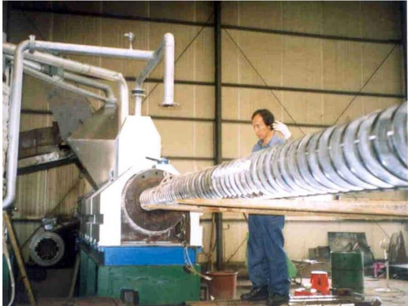
Fig. 3-6-11 Twin screw setting
