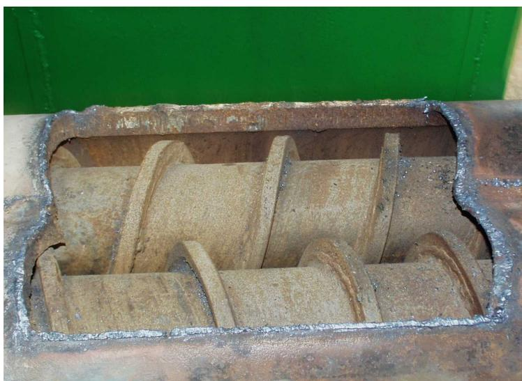
Fig. 3-6-17 Twin screw for discharging
