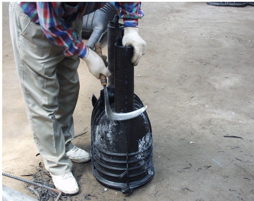
Fig. 3-6-34 Bur removing process
