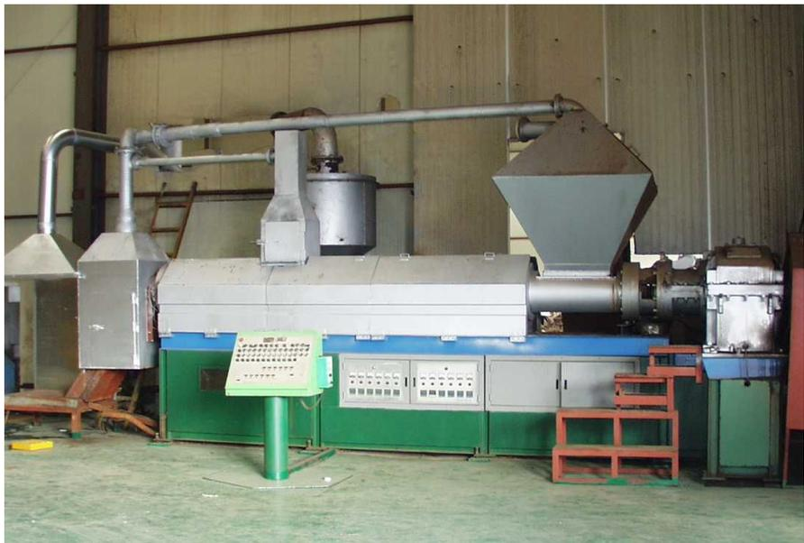
Fig. 3-6-27 View of modified electric heating type system
