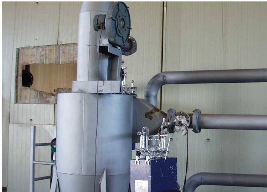
Fig. 3-7-1 Sampling point-1 (inlet of cyclone)
