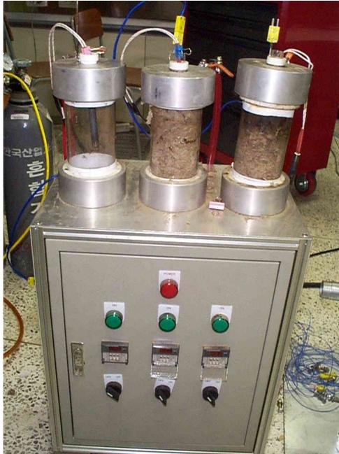
Fig. 3-5-11 Pyrolysis apparatus
